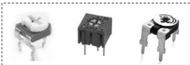
Some example of real life potentiometers
