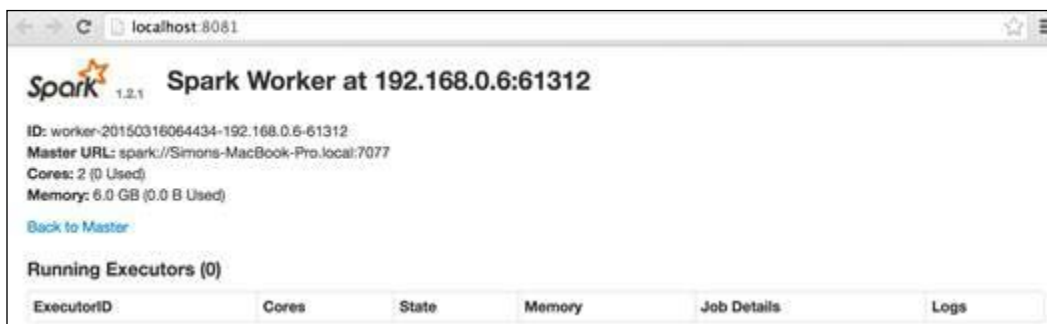
Figure 7: Worker's web monitoring console in its initial state with no application executors created.
