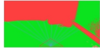
Now we can project lines from the center bottom of the image to the place where they encounter a red pixel. That is our safe driving zone
