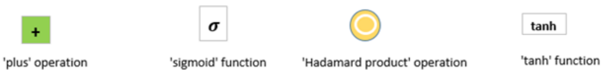
Figure 6.7: The meanings of the different signs in the GRU diagram
