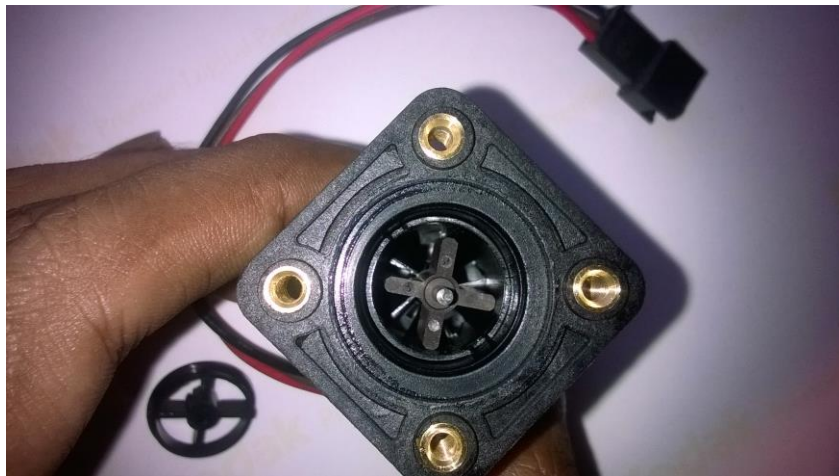
Pinwheel attached inside the water flow sensor
