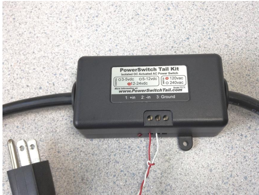
Two wires from Arduino is connected to the PowerSwitch Tail
