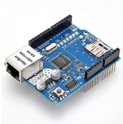
Arduino Ethernet Shield R3 (Front View)
