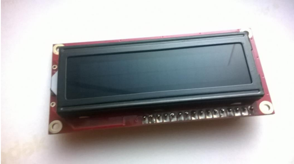
Hitachi HD44780 driver compatible LCD screen (16 x 2)—Top View
