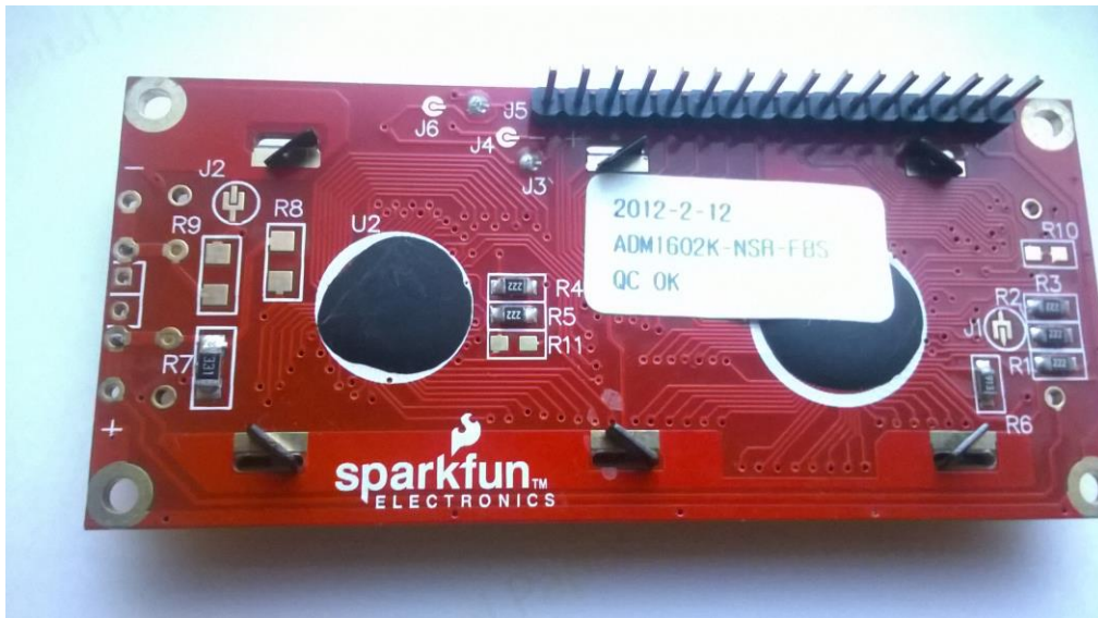
Hitachi HD44780 driver compatible LCD screen (16x2)—Bottom View
