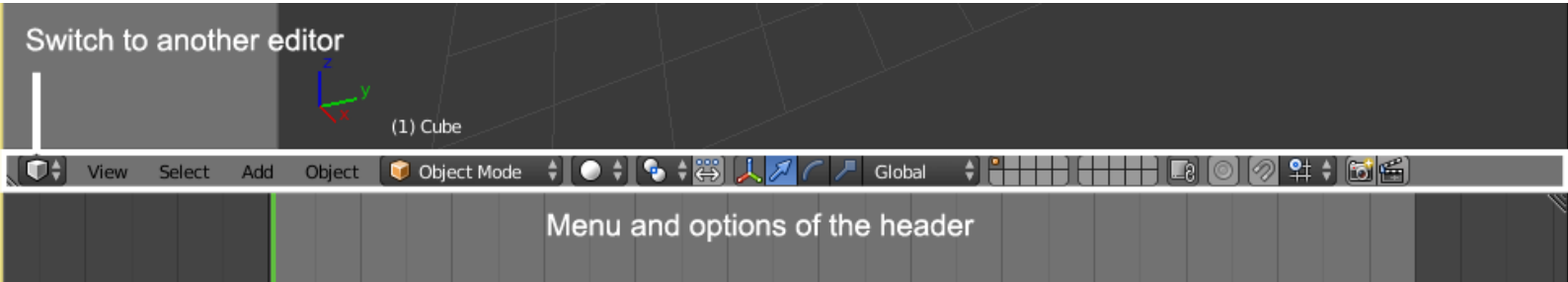
The header of the 3D View-port. The first button is for switching between editors, and also, we can switch between the menus and options
