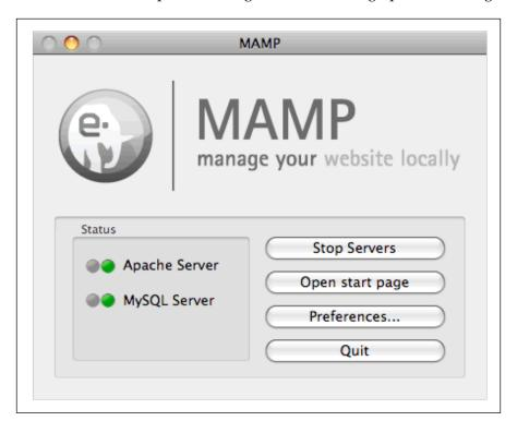
The preceding figure shows the main MAMP control, from where you can start and stop the server, and configure any settings related to the server environment.
