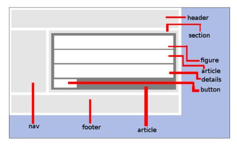
This is a wireframe of the structure we'll develop. Note that the article element directly inside the section tag is representative of a single game card widget. Thus, the entire structure it represents will be repeated for each game that we'll be showing off in our portal page.
