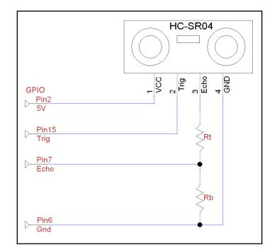
$$V_{out} = \frac{R_t}{(R_t + R_b) \times VCC}$$
