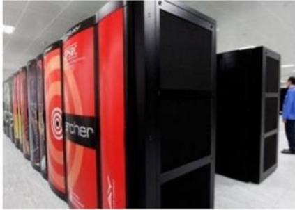
ARCHER has 4920 nodes in 26 cabinets giving a total of 118,080 cores
