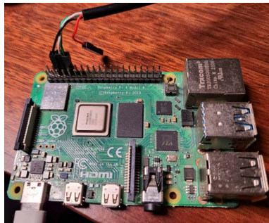
Figure 14.4: The Raspberry Pi 4 Model B with a USB-to-RS232 TTL UART serial adapter cable attached to its GPIO pins
